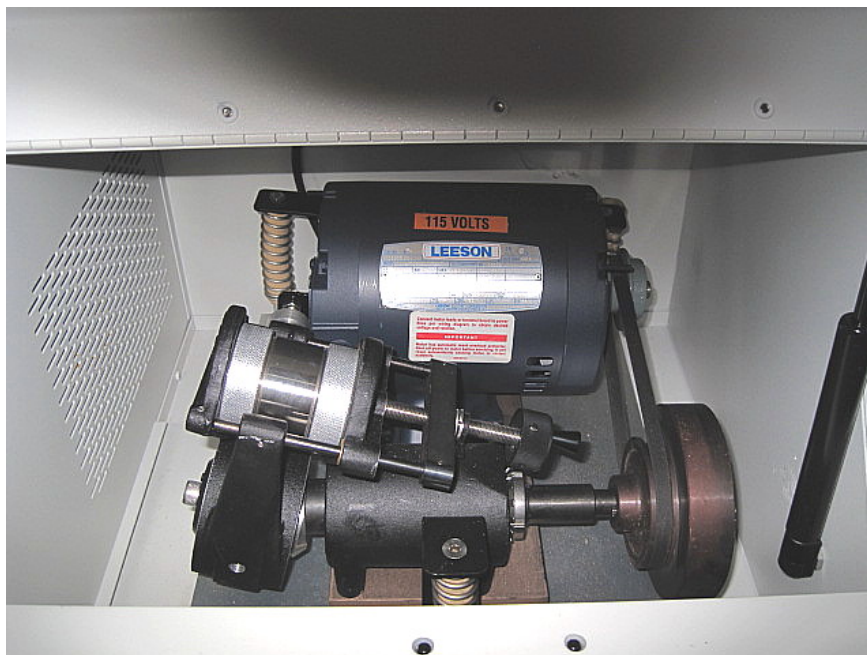
Figure 2.1. Spex Mill 8000 vibratory shaker mill.
